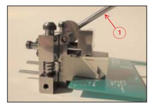
Place connector into the takeoff device for the organizer. By locking the latching device lever into position (see Fig. 2) clamp fast the connector in the takeoff device. By operating the lever (1) the top housing section (organizer) is shifted to the rear.
