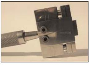
Adjustment with the arrester device screwed on. For pressing out contact wafers where the signal contacts do not protrude from the printed circuit board.
