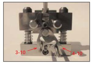
Two different latchings are possible. For the female connectors type 4-10 or 3-10. For type 2-10 there is a separate device..
