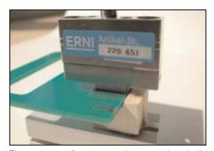
The contact wafers can now be pressed out individually by means of the manual device. The tool is securely fixed at the termination side by means of the signal contacts. There are two adjustment possibilities on the tool to ensure a secure fixing (depending on the thickness of the printed circuit board and the termination length of the signal contacts).
