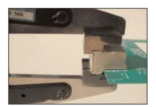
Now use the manual grippers to withdraw carefully the front section of the housing.
