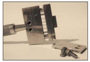
Adjustment with the arrester device screwed off. For pressing out contact wafers where the signal contacts do protrude from the printed circuit board.
